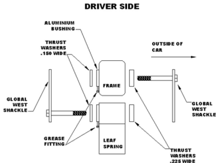
Using the ½ inch bolts supplied in your kit, finish assembling the shackle. You can install the bolts from the inside or outside, it makes no difference. Hang the shackles of the frame first and then slide the leaf up into position. Install the locking nuts.
