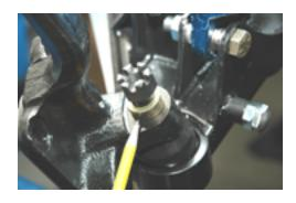
12. Install the upper ball joint through the spindle. Torque the upper ball joint to 70-foot pounds and cotter pin.
