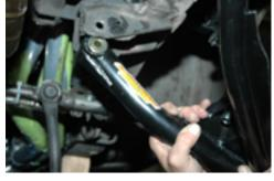
adjuster so there are approximately two threads showing on each side of the jam nuts. Feel the amount of pressure needed to adjust the wrench. What you are looking <u>for is the least amount of resistance to move the wrench / hex adjuster</u>. If you adjust the length too long or short, the rod end will have unnecessary side loads placed on the bearing and you will feel that when you are adjusting the assembly. The hex adjuster is harder to turn.
