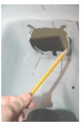
The new shock mount has a machined groove cut out to allow the tabs to rest inside the mount. Sometimes the tabs require a slight bend so they will fit into the mount. You do not have to grind these tabs, simply bend the tabs using a pliers. The goal is to have the mount seat flat up against the tower.
