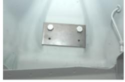
Drill the new hole location with a 3/8 drill bit and then step the hole up to a final size of 9/16 diameter.
