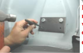
If you have ordered a nonnegative roll system (ST) you will still need to drill the original holes out to 9/16 diameter.
