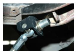
Slide the other side of the lower a-arm up into the frame. Occasionally due to frame
