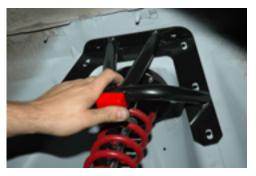
Install all the bolts and nuts in the support loosely. Place the head of the bolt in the engine compartment side. Tighten down the top 2 bolts first and then move from the top, side bolts down the bracket. Tighten to 25 pounds.
