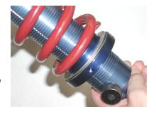
E. Next locate one spring adapter ring. The ring will index on top of the spring.
