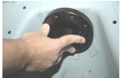
3. If you have ordered a negative roll system you will have an upper control arm template for drilling different locating holes. Note: If you did not order a negative roll
