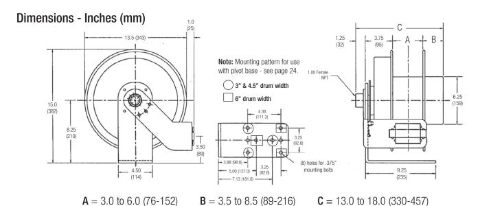
A, B, and C dimensions depend on the exact reel configuration - Contact Factory
