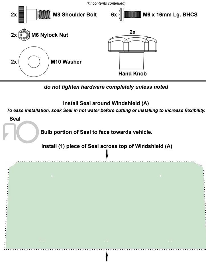
install (1) piece of Seal to sides and bottom of Windshield (A)
