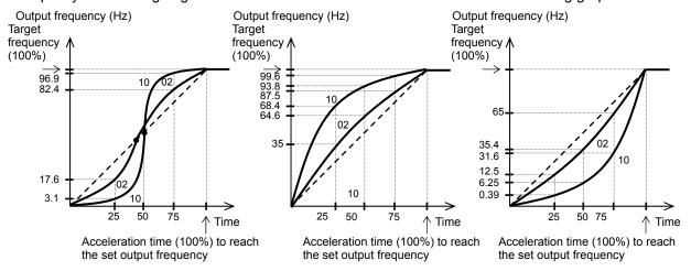
The acceleration or deceleration time may be shortened midway through the acceleration or deceleration according to the S-curve pattern.
