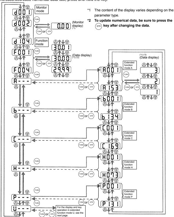
(3) Code/data display and key operation in extended function mode U
