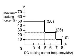
DC braking force limiter(90-160kW)
