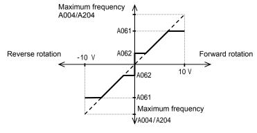
If the frequency lower limit is used with the frequency command input via the O2-L terminal, the motor speed with 0 V input will be fixed to the frequency setting of the frequency lower limit (A062) for forward rotation or the frequency setting of the frequency lower limit (A062) for reverse rotation as shown below.
