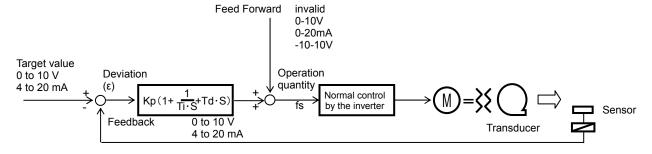
Kp: Proportional gain Td: Derivative time Ti: Integral time s: Operator : Deviation
