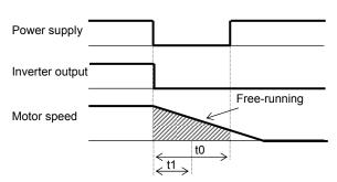
(Example 3) When the motor frequency (speed) is more than the setting of "b007":
