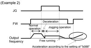
When "03", "04", or "05" is specified for the jog stop mode (A039), the jogging operation will be performed, even if the FW signal is turned on earlier than the JG signal. However, the motor will stop after free-running if the JG signal is turned off earlier than the FW signal.
