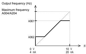
If 0 V or 4 mA is input as the frequency command when a frequency lower limit has been set for the frequency lower limit setting (A062), the inverter will output the set frequency.
