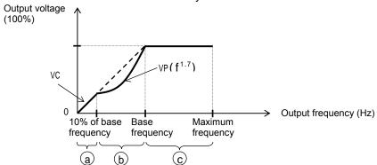
Period (a): While the output frequency increases from 0 Hz to the 10% of the base frequency, the output voltage follows the constant torque characteristic.
