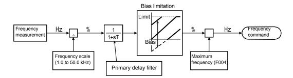
Block diagram for pulse train frequency input
