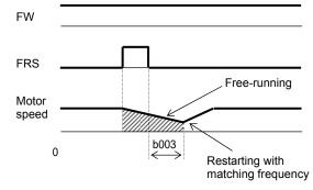
The inverter waits for the retry wait time after the FRS terminal has been turned off, detects the motor speed (frequency), and restarts the motor with the matching frequency without stopping it. If the inverter trips because of overcurrent when it restarts the motor with matching frequency, prolongs the retry wait time.
