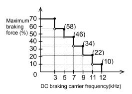
DC braking force limiter(11-75kW)
