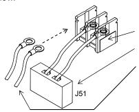
Remove the connected cables.
