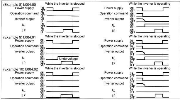
Note 1: You can assign the instantaneous power failure alarm signal (IP: 08) and the undervoltage alarm signal (UV: 09) to any of the intelligent output terminals [11] to [15] (C021 to C025) and the alarm relay terminal (C026) to output the alarm signals.
