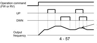
Turning on the UP and DWN terminals at the same time disables acceleration and deceleration.
