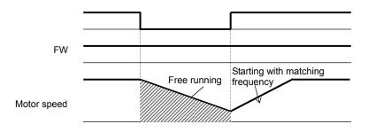
Note: The reset operation clears the inverter's internal counters that are used for protective functions. Therefore, if you intend to use an intelligent input terminal to shut off the inverter output, use the free-run stop (FRS) terminal.
