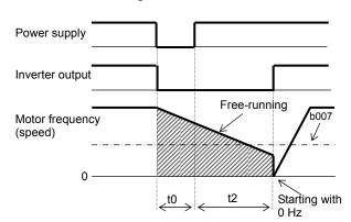
(2) Output of the alarms for instantaneous power failure and undervoltage in the stopped state Use function "b004" to specify whether to output an alarm when instantaneous power failure or undervoltage occurs.
