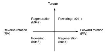
When "01" (terminal-switching mode) is specified for the torque limit selection (b040), the torque limits 1 to 4 are set as shown in the example below. The torque limits 1 to 4 are switched by the torque limit switches 1 and 2 assigned to intelligent input terminals.
