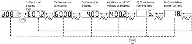
\*2 If the inverter has not tripped before, the inverter displays
