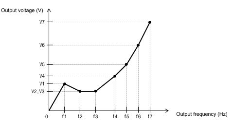
\*1 Even if 800 V is set as a free-setting V/f voltage (1 to 7), the inverter output voltage cannot exceed the inverter input voltage or that specified by the AVR voltage select.
