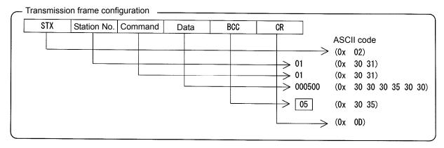
The contents of "Station No." to "Data" are converted into ASCII data, and the ASCII data is XORed bit by bit. The final XOR result is set as the block check code (BCC). In the above example of transmission frame, BCC is calculated as follows:
