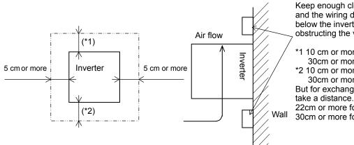
Keep enough clearance between the inverter and the wiring ducts located above and below the inverter to prevent the latter from obstructing the ventilation of the inverter.
