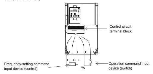
(3) Entering operation and frequency-setting commands; both from a digital operator and via control circuit terminals
