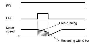
regardless of the motor speed. The setting of retry If the inverter restarts the motor with 0 Hz when the motor speed is high, the inverter may trip
