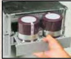
Easy-removable Dc bus Capacitors (SJ700: above 15kW L700: above 18.5kW)
