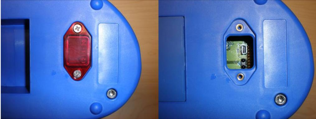
**Figure 7: USB/IR Cover Location and Cover Removal**
