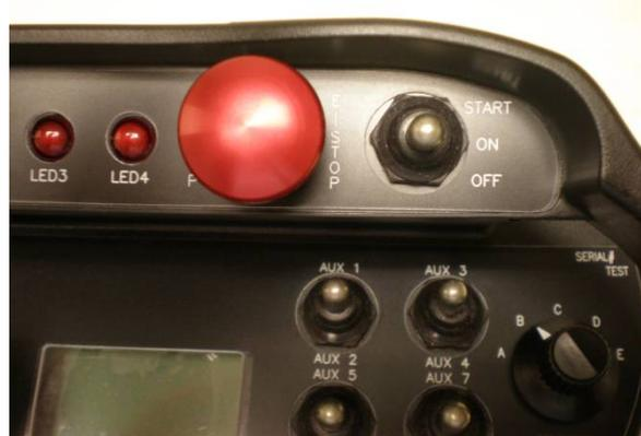
Figure 9: Machine Stop Switch and OFF-ON-START toggle
