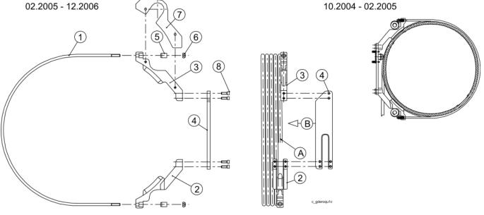
A Rope leaves the rope drum B Rope fixing clamp side
