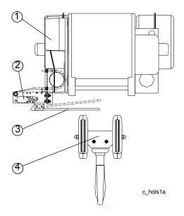
1.Hoist 2.Limit switch 3.Limit switch lever 4.Hook
