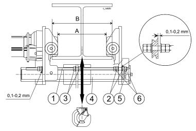
6.5.2 Curved beam, when two trolleys
