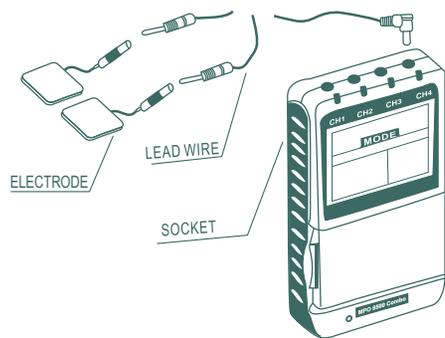
After connecting the wires to the stimulator, attach each wire to an electrode. Use care when you plug and unplug the wires. Jerking the wire instead of holding the insulated connector body may cause wire breakage.
