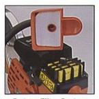
5-stage Filter System Ensures clean air supply even in dusty conditions
