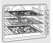
The oven has 5 shelf positions. Place the gray porcelain-coated racks in positions "R", "B" and "D" for self-cleaning the grates. Place one grate each on the oven racks from side to side.
