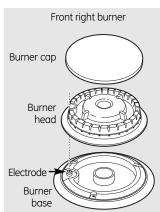
Make sure the hole in the burner head is positioned over the electrode and that the burner head is fully inserted inside the burner base. A small gap between the base and head is normal.
