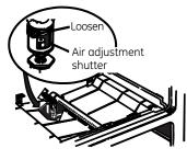
The shutter for the bottom (oven) burner is near the back wall behind the drawer. Remove the drawer. See the *Care* and cleaning of the range section.
