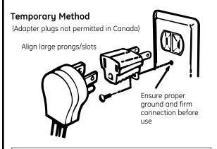
**CAUTION:** Attaching the adapter ground terminal to the wall receptacle cover screw does not ground the appliance unless the cover screw is metal, and not insulated, and the wall receptacle is grounded through the house wiring. The customer should have the circuit checked by a qualified electrician to make sure the receptacle is properly grounded.
