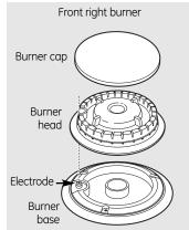
Make sure the hole in the burner head is positioned over the electrode and that the burner head is fully inserted inside the burner base. A small gap between the base and head is normal.
