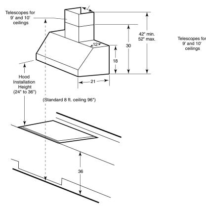
Installed above a range (shown with optional chimney kit) (Dimensions in inches)
