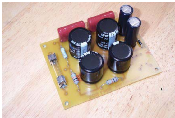
PAS Power Supply Capacitor Board
