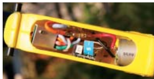
The receiver, speed control and motor are nested in the pylon that supports the main wing.
