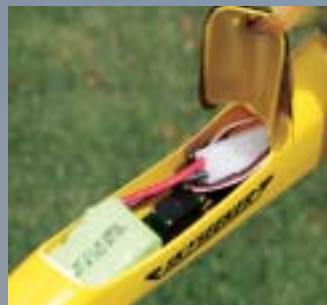
The 6-cell NiMH battery fits under the hatch in the nose of the plane. A rubber band holds the hatch down by gripping the exterior.
