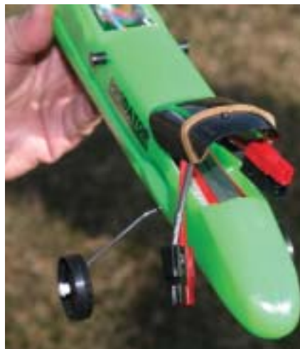
Top: The 1500mAh Kokam 7.4v Li-Poly pack fits nicely in the nose of the Predator. This pack offers slightly greater speed and twice the duration of the stock NiMH battery. Bottom: Extra props and rubber bands are included.
