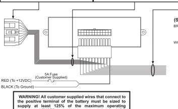
current and FUSED at the battery to carry that load. DO NOT USE CIRCUIT BREAKERS WITH THIS PRODUCT!
