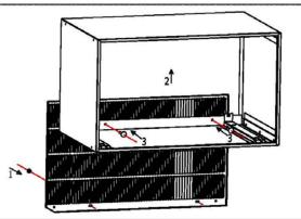
**4\***、As shown in picture 1, fix the grille fixed cap on the grille, insert the grille into the slot of the top cover as shown in picture 2,lock the bottom cover assembly and grille tightly with 2 pieces grille fixed screws as shown in picture 3.
