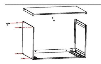
3. As shown in picture 1, install the top cover assembly on top of the left and right cover assembly, and then lock them tightly with screws as shown in picture 2.
