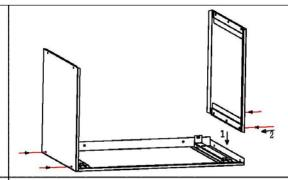
2. As shown in picture 1, insert the left cover assembly and right cover assembly on the bottom cover assembly, and then lock them tightly with screws as shown in picture 2.
