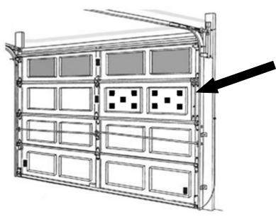
**Practice/Step 1:** It is best to use the extra size of the panel to help hold the panel in place. Simply "push" and "move" the panel in the proper position within the panel to the desired fit (*before using the adhesive squares!*) The panels can be trimmed but *only* if necessary. Once you "see" how the panels will fit proceed to the next step.
