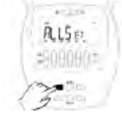
Fig 13b – Press and hold the INCLUDE button
