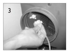
Connect the female half of the quick connector at the end of the spiral water pipe to the male part in the hot air outlet pipe.
