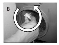
Only Required For Disassembly. In order to unlock the quick connector, push the tab and turn the connector counter-clockwise.
