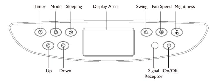
When plugging in, follow the start music until the unit is in standby status. The digital screen will indicate the temperature (Range: 41°-95°F), if the temperature is above 95°, the screen will show "H", if below 41°, it will indicate "L".
