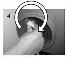
Turn the connector 90 degrees clockwise until it is locked in place.
