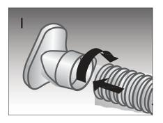
Attach Window Slide Bar Connector to Exhaust Hose by twisting as shown.
