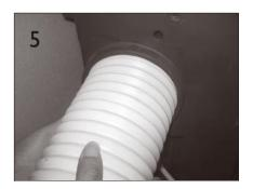
Assemble the hot air hose on the unit.
