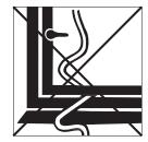
Where the power cable may be damaged
