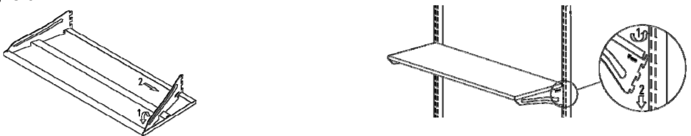
Fig. C-3 Metal Shelf Bracket installation and hanging installation
