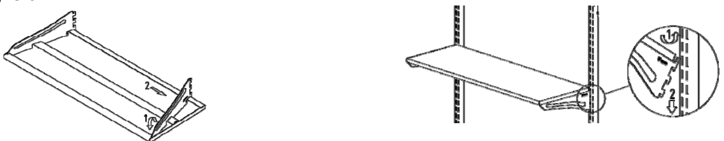
Fig. C-3 Metal Shelf Bracket installation and hanging installation
