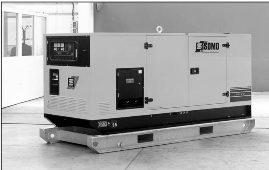
Fig. 1-1 Small modular units need little space and take very little time to install. This JS 100 Euro Silent generation package is equipped with a John Deere 4045 HF 157 Powertech engine. It generates 100 kWe with relatively little noise – 70 dBA at 23 feet.
