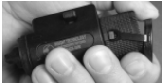
Push Filter Away from Bezel with the Thumb
