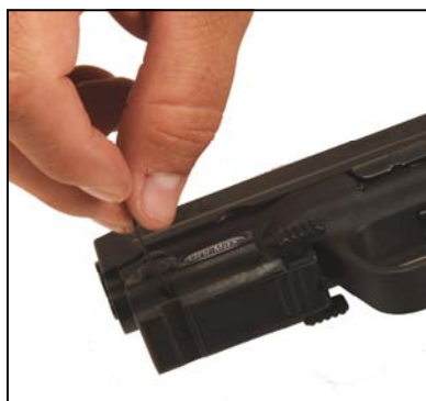
The hole at the side adjusts windage (horizontal alignment).
