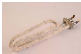
<Inside of Boiler w/limescale build-up
