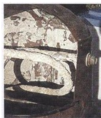
<Inside of Boiler w/limescale build-up
