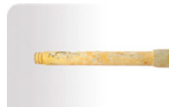
<Boiler heating element w/limescale
