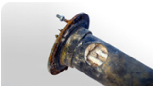
<Inside of Boiler w/limescale build-up
