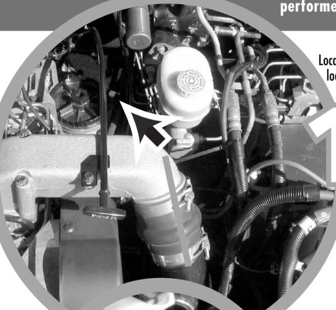
1 Locate your MAP sensor located on the right side of the engine block
