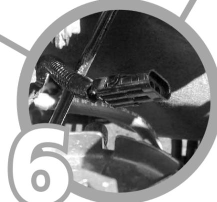
6 Connect the DiabloSport PowerPuck male Data Link Port connector into the engines Data Link Port.
