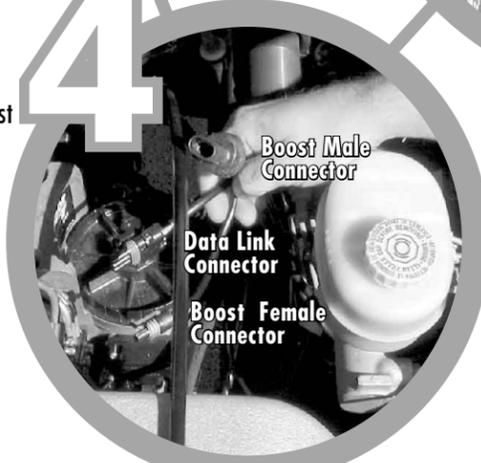
4 Connect the female connector of the boost control cable to the MAP sensor.
