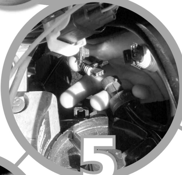
5 Locate you Data Link Port Connector, remove the cap covering the port.
