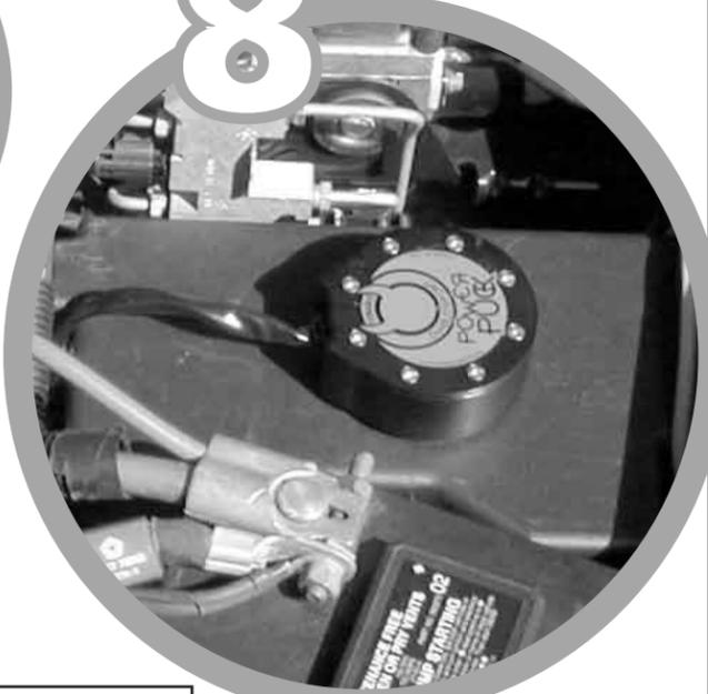
8 Carefully peel off the Velcro protective film and firmly affix the PowerPuck in place. Let it dry for 24hrs before removing Puck.
