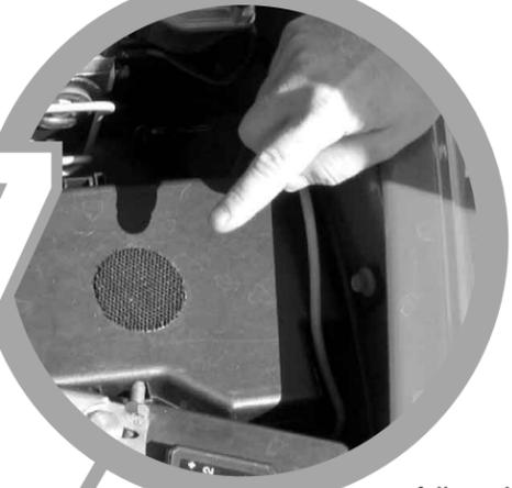
7 The PowerPuck will find its home on top of the fuse box cover. (this will allow for quick and easy access) Clean the top of the fuse box with the alcohol pad provided. Wait for the alcohol to dissipate.
