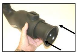
12. Install the Modular Venturi Tube (MVT) (#3) into the Airaid Intake Tube (#2) as shown. Option: For additional air flow, delete the MVT. This requires custom computer programming. Engine damage will result without the use of custom tuning. (SEE #22 BELOW!!)
