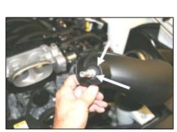
**11.** Install the supplied grommet (#15) and aluminum fitting (#18) into the Airaid intake tube as shown.
