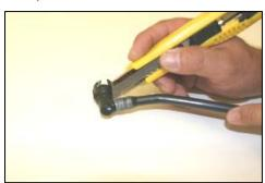
**17.** <u>VERY CAREFULLY!</u> With a razor blade, cut the plastic tube off both of the factory breather hose ends as shown.
