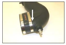
**14.** Install the oval coupler (#4) with two #72 hose clamps (#13). Tighten only the clamp closest to the aluminum fitting. (*Hint:* For a clean look, locate the tightening screws under the tube)!
