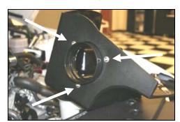
**8.** Install the air filter adapter (#6) into the Cool Air Dam (#7) as shown, using 3 button head bolts (#10) and ½" flat washers (#11).
