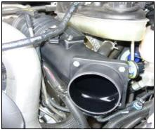
10. Slide the Airaid filter tube into factory flexible turbo inlet hose. (Note: Do not tighten hose clamp until assembly is complete.) Reconnect the sensor to the factory plug. (Either the temperature sensor or the mass air sensor, which ever you have.)
