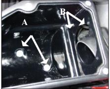
**12.** *A.*) Insert the supplied billet rivets thru the airbox, into the factory grommets. *B.*) Using 4 supplied stainless steel ½-20 Allen bolts and washers, mount the air filter tube to the airbox.
