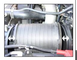
2. Remove factory air filter by separating the inlet and outlet sections of the assembly.
