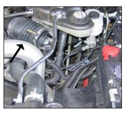
7. Remove complete factory air filter tube assembly. (Note: do not remove flexible turbo inlet hose from turbo housing.)
