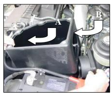
**11.** *A.*) Install the Airaid Cool Air Box by inserting the long extension of the box into the radiator support. (*Note: Make sure the cold air box inlet is not blocked by factory insulation.*) *B.*) Insert air filter adapter into air box hole.
