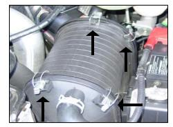
**1.** Disconnect both negative battery cables. Unlatch all four factory clips on the factory airbox.
