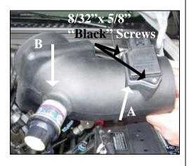
**9.** *A.*) If you have the sensor shown in step # 6, install the gasket and sensor using 2 (*black*) 8/32"x 5/8" screws. *B.*) Install the factory grommet and filter restriction gauge.
