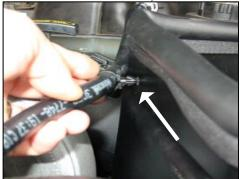
**18.** Spread the supplied hose mount over the radiator overflow hose and insert the tab thru the hole in the side of the panel.
