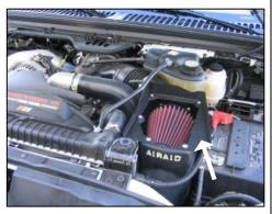
**16.** Install the black panel onto the top of the airbox using the 5 supplied stainless steel ½-20 Allen bolts and washers.
