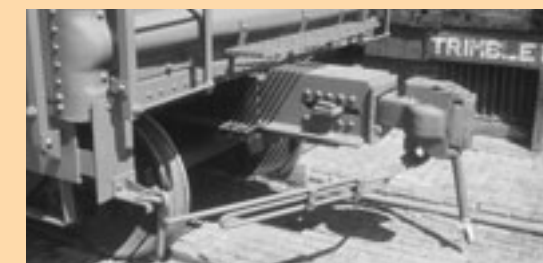
The draft gear on cushion underframe cars extends from the body, allowing for spring travel as the coupler and draft gear travel in and out. Linn Westcott
