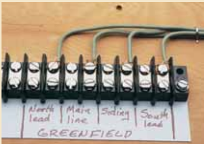
6 Terminal strips. Barrier terminal strips keep the loose stands of wire from touching each other.
