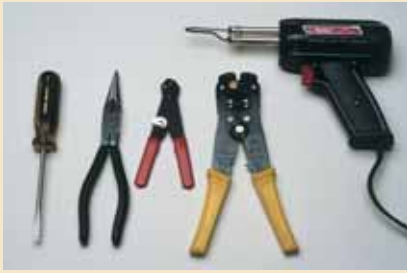
1 Tools. Small and large (6" and 8") wire cutters and a combination wire stripper/crimper are vital for working with wire.
