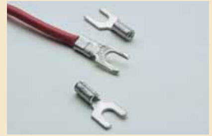
3 Solderless connectors. Use the crimping tool (a special pliers) to permanently crimp solderless connectors onto the ends of wires.
