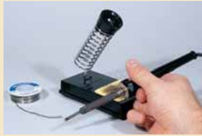
2 Soldering iron. A 30-watt pencil-type iron with stand and rosin-core solder will handle most soldering jobs on your model railroad.
