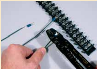
5 Crimping. Attach solderless connectors to wire by threading them onto the stripped end and crimping them in place.
