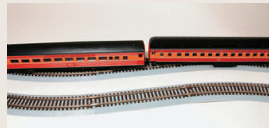
B Long cars won't operate well on S-curves. A section of straight track added between the curves will help smooth operations.
