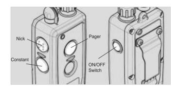
The transmitter for the **dogtrd** 2300NCP Advance single dog unit has four buttons (one on the face of the transmitter, two on the left side and one on the right side).
