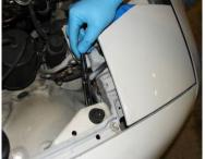
Step 3) Now it is time to remove the first vertical 14mm nut. It is located right behind the headlight while the headlight is in the closed position. Use a socket wrench with an extension on it to reach it,
