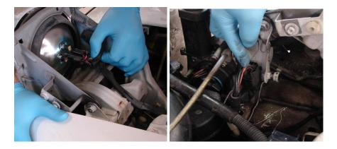
Steps 9) After both plugs have been removed unsnap the factory harness, which is held by small clips to the headlight assembly itself. Once those are removed the entire assembly can picked up and removed from the car. The end result will look like this.
