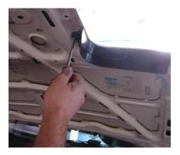
Step 5) Now it is important to check for fitment of all pieces. After everything is fitted to your desired result you are now able to drill the holes for your bucket. I would recommend either drilling the holes while the bucket is on the car or to take careful measurement. If you do not plan to ever run the clear covers your measurement will be slightly different then if you want to run the covers.
