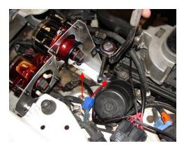
Step 4) Find one of the included locking washers and nuts. First screw the nut on the bolt as far as it will go and then install the locking washer. It is now time to slide the last mounting hole through the bolt until it reaches the locking washer. Install another locking washer and then the last nut. You will need to tighten down the bolts with a 13mm socket and wrench.
