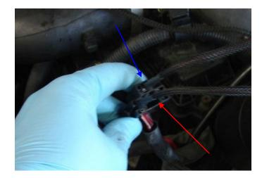
After everything has been plugged in you can now test the lights before you actually install them. Find the longer set of connectors and run them on the back of the firewall to the passenger side of the headlights.
