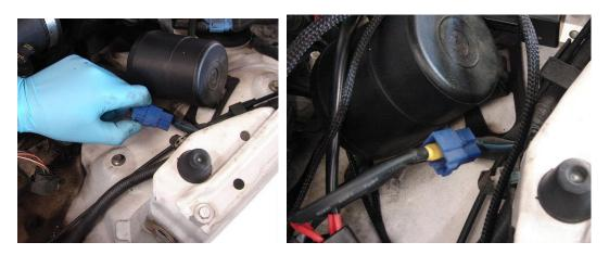
Step 3) Find the ground wire, it is a black loom with an o-ring terminal on the end. Right below the blue connector there is a 10mm bolt on the bottom portion of the fender well hump. Unbolt this bolt and ground the wire here. In order to assure a good ground you should use sandpaper to remove the paint and grease where the terminal will contact the chassis.
