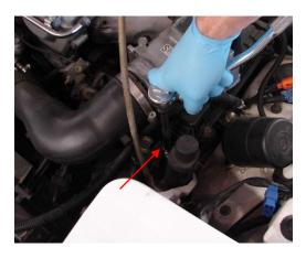
Step 2) After the bolts are removed you can now unscrew the hose clamp and move the plastic intake elbow out of the way.
