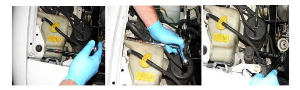
Step 2) with the overflow bottle out of the way it is now time to remove the first nut. This nut is positioned horizontal in relation to the car and was hidden behind the overflow bottle. With a socket wrench remove this 14mm nut.
