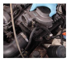
Step 3) Now that the elbow and box itself are out of the way, there is plenty of room to use a 14mm open or box end wrench to remove the last vertical nut.
