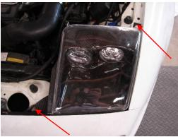
Step 7) on the back of your factory headlights is your prop rod and connector for it. Remove both of those pieces from your factory headlights. On the rear of each metal bracket is a tab with a hole in it. Snap in the prop rod to one and the connector to the other.
