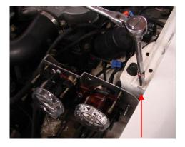
Step 2) The Carbon Fiber buckets have 3 mounting points. The addition of the front "leg" is used for support and is not bolted to anything. When you try and install the bucket make sure to slide the rear of the cover on first and then push the leg of the bucket into place. The fit is tight so take your time and make sure it is done right. In order to get
