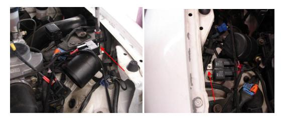
Step 2) Now it is time to connect the 12v power source. With the fuses removed, find the blue plug on the driver side of the engine compartment. Unplug the cover and insert the yellow power plug over the connector.
