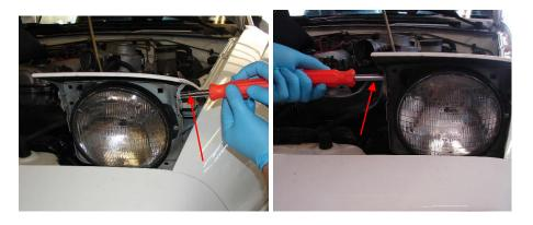
Step 8) After you have successfully removed the headlight lid you can now proceed to unplug the harness from the back of the headlight. Once the harness is unplugged, in order to remove the headlight from the car another connector next to the headlight motor
