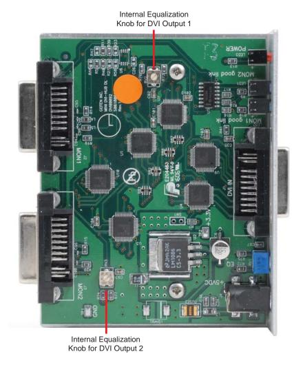
The internal E.Q. knobs can be reached by removing the 6 hex nuts on the DVI connections and the 4 screws on the bottom of the unit.
