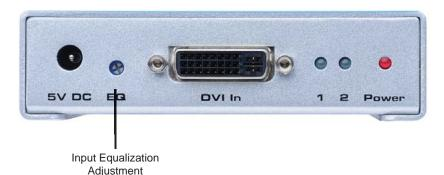
The external equalization knob can be used to balance out signal noise resulting from long cables for better picture quality. By turning the equalization knob counter-clockwise you will eliminate any noise and/or degradation in the signal. You should be able to find a "sweet spot" somewhere in the middle.
