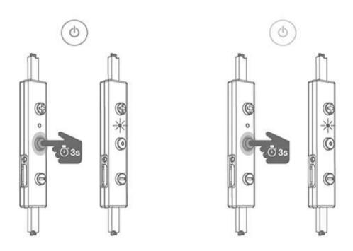
To power on your BE6, press Power/Function button for about 3 seconds until the LED indicator flashes blue and you hear the "Power on" when voice prompt is activated or a beep if the voice prompt is not used.
