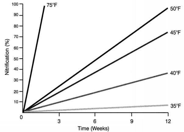
FIGURE 4-2. Generalized nitrification rates at various soil temperatures.
