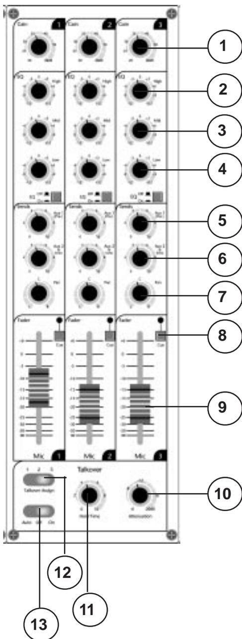
1. **Gain:** This controls the input level for the “LINE” and “XLR” microphone inputs for the channel. It can be adjusted from 20dB to 60 dB.
