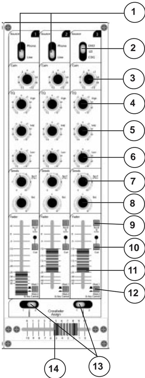
1. **Source Selector: Channels 1 and 2** allow the user to connect two players **without** video output. The source selector switch makes it possible to switch easily between players by “toggling” it to the desired position.
