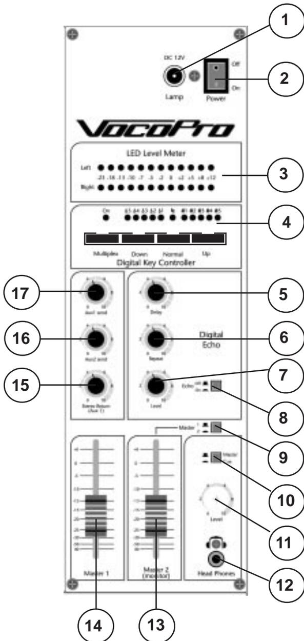
4. **Digital Key Control & Multiplex:** The digital key control feature works in the Master 2 mode. Press the Master 2/Key Control button on the desired channel (to the down position) then adjust the key control up or down to raise or lower the “key” of the music. **The Multiplex feature works only with discs recorded in the “multiplex” format. It will delete the vocal tract on multiplex CD’s or tapes.**
