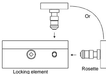
When the door is closed, the locking bolt of the rosette engages the locking element and the safe-deposit is locked. If the safe-deposit must be opened, the compact locking element must be unlocked electrically first.
