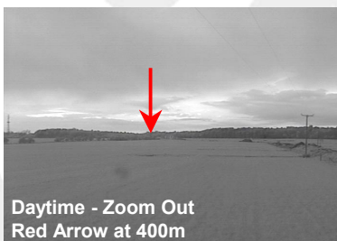
Daytime, Zoom Out: An overview image of a distant scene. The red arrow indicates a distance of 400m (1,300ft), where no details are visible, even during daytime.
